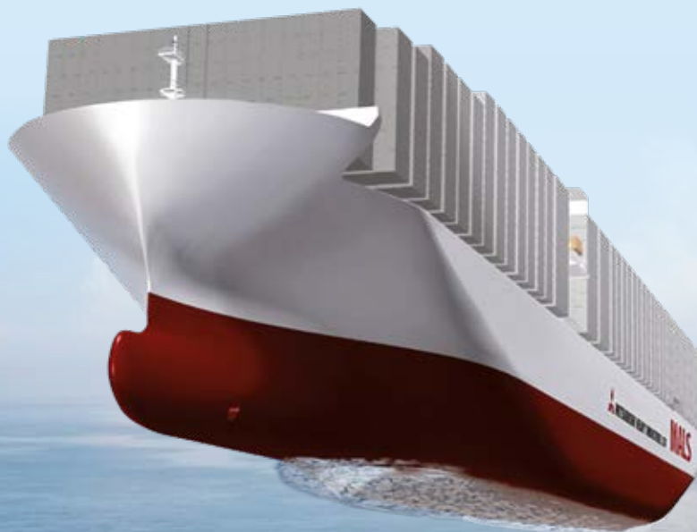
AERZEN ALS technology (Air Lubrication Systems): if process air is blown under the bottom of a ship's hull, this reduces friction between the ship's hull and the surrounding water and thus reduces fuel consumption.
