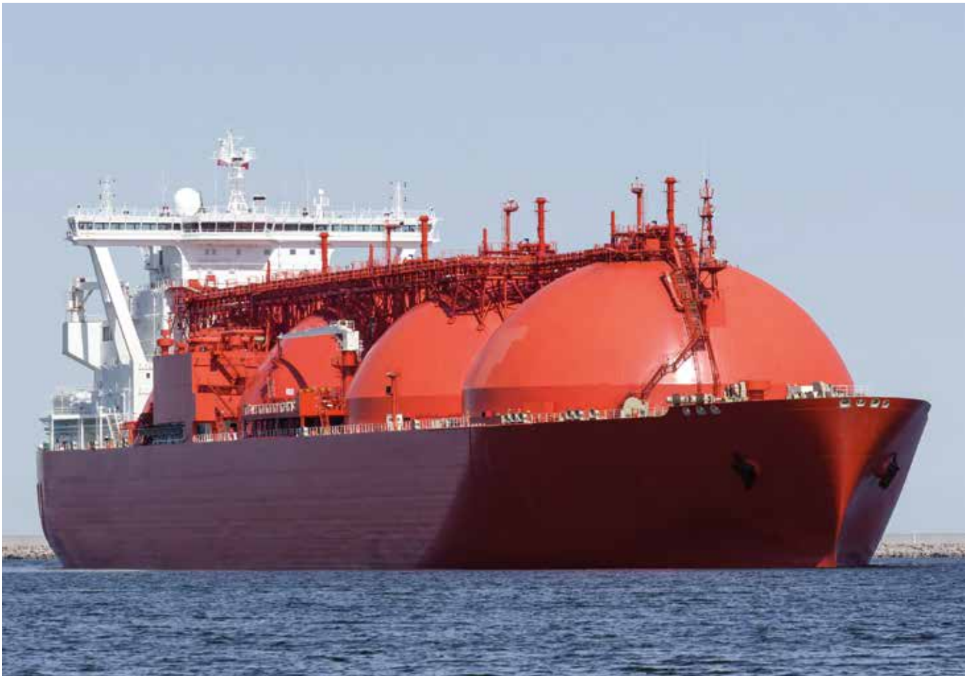
AERZEN compressors can feed the boil-off gas, which is produced on LNG tankers during transport by heating LNG, back to the ship's engine after pressure adjustment.
